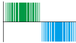
Two level output voltage waveform
