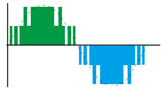
Three level output voltage waveform
